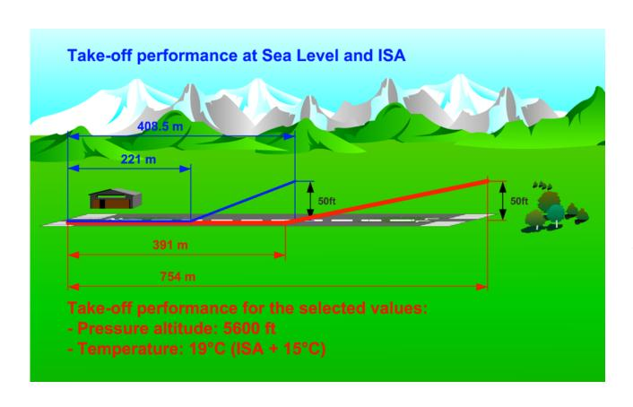
Higher density altitude means thinner air which seriously degrades aircraft performance.
