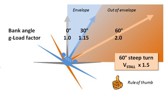
**Stall speed:** As weight doubles (60° bank), stall speed increases by V2, or 1.414
